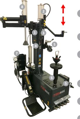
Easy Demount Head (Upper Bead): Bead controls up and down and the bead is demounted.
